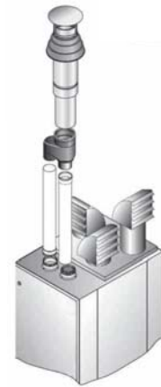
Balanced flue roof outlet (type C32)
